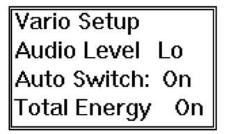
This is how the **Vario Setup** page appears when you turn to it. It is a **list page**, which means that there is more information than will fit in the display at one time. Use the **==>** key to move the cursor and scroll the display.
